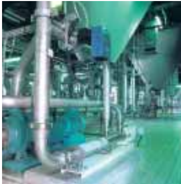
13IA12 in animal feeding for transferring and injecting ingredients (oils, molasses, enzymes, etc.).
