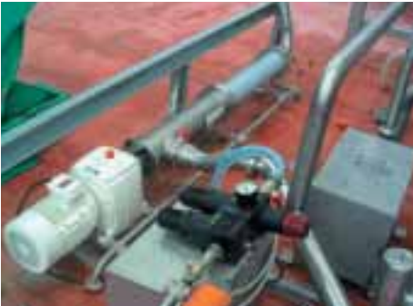
13IA12 in animal feeding for transferring and injecting ingredients (oils, molasses, enzymes, etc.).
