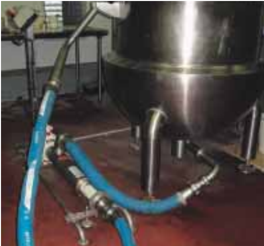
13IA6 in the sauce industry: transfer of ketchup or mayonnaise from the cooking phase to the storage tank.
